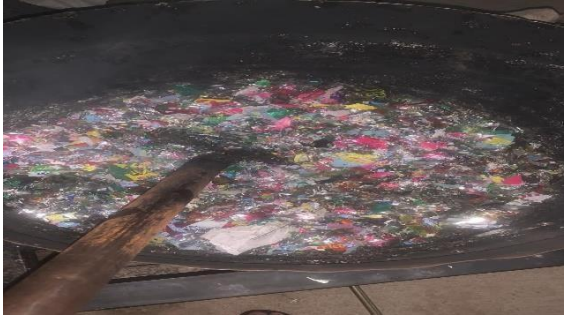
Gambar 4. 4 Proses Pelelehan Plastik
