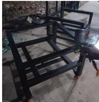
Gambar 3. 42 Proses Pengecatan Zink Chromatte
