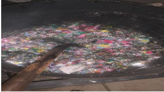
Gambar 4. 4 Proses Pelelehan Plastik
