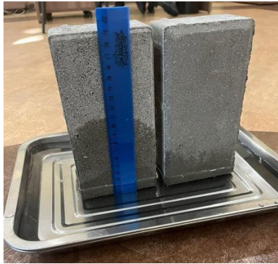
Gambar 5. 1 Ilustrasi Daya Serap Eco Paving Block
