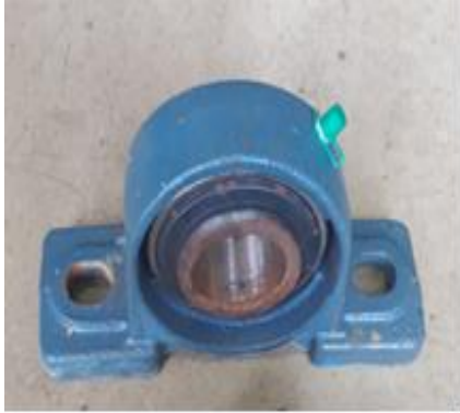
Gambar 3. Bearing tipe pillow block
