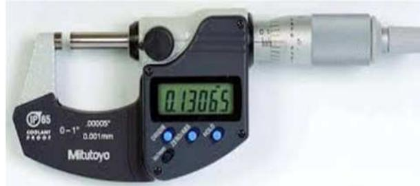
Gambar 35. Mikrometer digital
